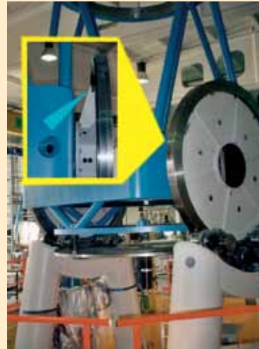
Perfect overshoot protection for precision telescope
