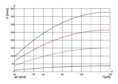
The curves indicate the volume flow through the complete filter system (filter housing including cartridge) and are referred to a differential pressure of 0.3 bar. Specific process information is essential to guarantee reliable operation of an
