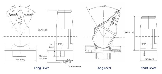
Joystick fitted with 2 x M3 inserts Maximum screw penetration 6 [0.236]
