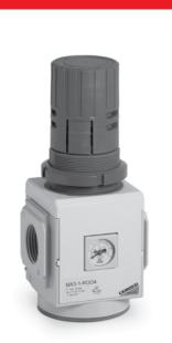
The availability of constant values of the secondary pressure ensures performance optimization and energy saving. The tamper-proof system allows to adjust pressure safely through 2 intervals with primary pressure compensation. All regulators are equipped with an integrated locking system and built-in pressure gauges for a more compact product. The regulators Series MX are suitable also for panel mountings.
