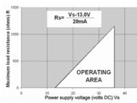
E.g. with supply voltage load of 36vdc, maximum load is 1150ohms
