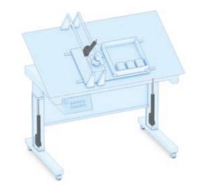
Placing the Electrak HD with synchronization into your ergonomic applications ensures a stable, effective lift for off-center or awkward loads.
