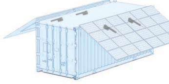
The Electrak HD is an industrial solution that can handle heavy loads - such as large solar panels - in rugged installations. These heavier loads, which would typically require structural support and larger actuation solutions, can be easily lifted with multiple HD actuators in sync.
