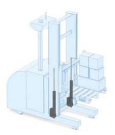
Applications using automation can benefit from internal condition monitoring with every HD actuator. This keeps the actuators running within rated specification and shuts them down if temperatures rise, loads are exceeded or input voltage is insufficient.
