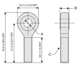
The rod end front adapter comes in one metric and one inch version. The metric adapter can be mounted to the front of the extension tube if the actuator is equipped with the metric female thread front adapter option (type P), while the inch adapter requires the inch female thread option (type G).
