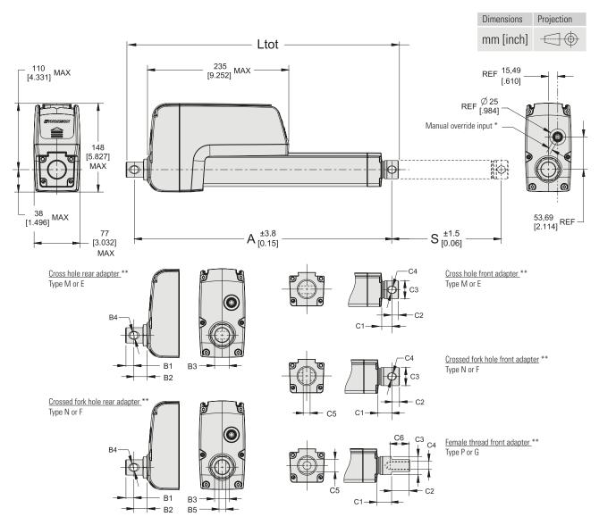
Manual override input. The input hole is covered with a plastic threaded plug. When removed, a 6 mm socket can be inserted and used as a crank.
