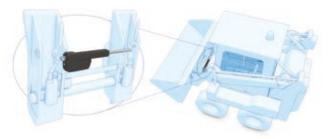
Quick-attach actuators allow the operator to change implements on the loader or skid steer without leaving the seat for improved productivity and safety.
