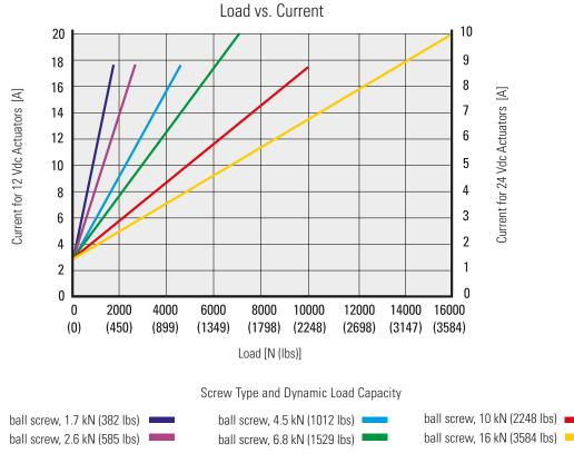
Note! Curves were generated at an ambient temperature of 21°C (70°F). Different ambient temperature and individual actuator characteristics can produce slightly different values.
