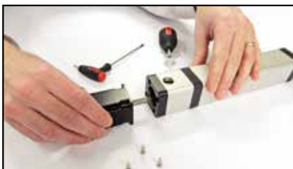
Insert motor shaft into coupling
