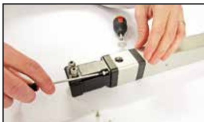
Tighten motor mounting screws
