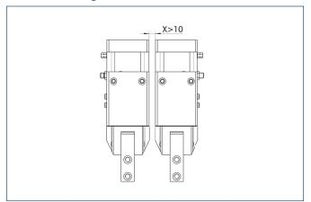
CAUTION: Monitoring is carried out by magnetic switches, and in case of side-by-side assembly of several units, a minimum distance of X mm between the units must be maintained.
