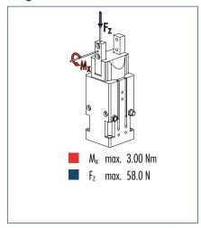
The indicated moments and forces are statical values, apply for each base jaw and should not appear simultaneously. If the maximum admissible finger weight is exceeded, throttling is necessary in order to ensure a smooth jaw motion without jerks or bounces. The life-time may reduce.
