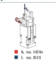
The indicated moments and forces are statical values, apply for each base jaw and should not appear simultaneously. If the maximum admissible finger weight is exceeded, throttling is necessary in order to ensure a smooth jaw motion without jerks or bounces. The life-time may reduce.
