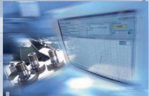
Computer-aided test stand for torque and engagement speed.
