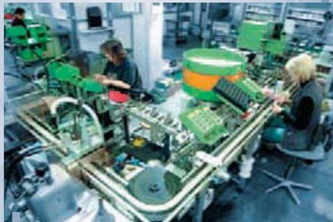
Assembly and testing of pressure switches on partially or fully automated plant.
