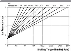
Minimum Pressure for full retraction: 5 bar Maximum Braking Force full rate: 6.4kN Weight of MR caliper and thruster - 10.0kg Weight of MR2 caliper and thruster - 10.5kg
