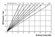
Maximum Pressure 100 bar Maximum Braking Force = 45kN @ 100 bar Weight of caliper - 18.6kg Volume displacement per 1mm stroke at each pad = 15ml
