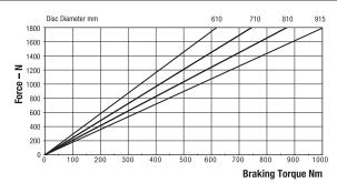
Weight of caliper and hand wheel assembly - 10.52kg Weight of hand wheel assembly only - 1.3kg Maximum Braking Force = 2.68kN
