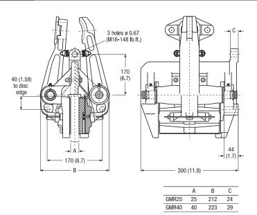
The Twiflex GMR and GMR40 series of disc brake calipers is suitable for use with discs of 25.4mm, and 40mm thick respectively. Minimum disc diameter is 610mm.
