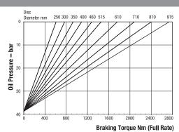
Minimum Pressure for full retraction: 50 bar Maximum Braking Force full rate: 6.4kN Weight of MR caliper and thruster - 10.5kg Weight of MR2 caliper and thruster - 11kg
