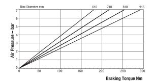
Maximum Pressure 7 bar Maximum Braking Force = 0.74kN @ 7 bar Weight of caliper and thruster - 9.56kg Weight of thruster only - 0.34kg Volume displacement of thruster at full stroke = 25ml
