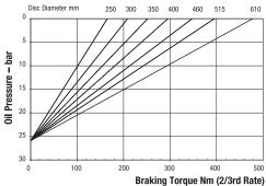
Maximum Braking Force 2/3rd rate: 1.74kN Minimum Pressure for full retraction: 33 bar Weight of caliper and thruster - 5.5kg Weight of thruster only - 4kg Volume displacement of thruster at 4mm retraction = 5ml
