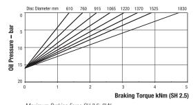
Maximum Braking Force SH 2.5: 6kN Minimum Pressure for full retraction: 21 bar Weight of caliper and thruster - 47.9kg Weight of thruster only - 13.9kg Volume displacement of thruster at full retraction = 56ml
