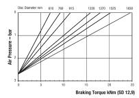
Maximum Braking Force SD 12.9: 30kN Minimum Pressure for full retraction: 3.8 bar Weight of caliper and thruster - 54kg Weight of thruster only - 20kg Volume displacement of thruster at full retraction = 2.5 l
