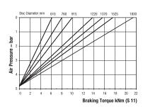
Maximum Braking Force S 11: 25kN Minimum Pressure for full retraction: 6 bar Weight of caliper and thruster - 47.2kg Weight of thruster only - 13.2kg Volume displacement of thruster at full retraction = 1.3 l
