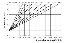
Minimum Pressure for full retraction: 65 bar Maximum Braking Force XSH 7.5: 11.2kN Weight of caliper and thruster - 11.4kg Weight of thruster only - 4.4kg Volume displacement of thruster at 6mm retraction = 9.1ml
