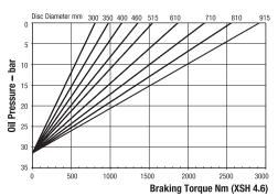
Minimum Pressure for full retraction: 40 bar Maximum Braking Force XSH 4.6: 6.8kN Weight of caliper and thruster - 11kg Weight of thruster only - 4kg Volume displacement of thruster at 6mm retraction = 9.1ml
