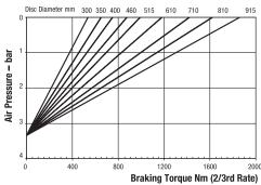
Minimum Pressure for full retraction: 3.3 bar Maximum Braking Force 2/3 rate: 4.3kN Weight of caliper and thruster - 10.5kg
