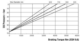
Maximum Braking Force XSH 9.6: 14.3kN Minimum Pressure for full retraction: 82 bar Weight of caliper and thruster - 13.82kg Weight of thruster only - 4.6kg Volume displacement of thruster at 6mm retraction = 9.1ml
