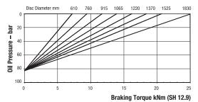
Maximum Braking Force SH 12.9: 30kN Minimum Pressure for full retraction: 100 bar Weight of caliper and thruster - 52kg Weight of thruster only - 18kg Volume displacement of thruster at full retraction = 56ml
