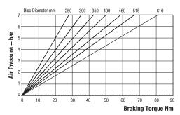
Maximum Pressure 7 bar Maximum Braking Force = 0.29kN @ 7 bar Weight of caliper and thruster - 1.91kg Weight of thruster only - 0.41kg Volume displacement of thruster at full stroke = 8ml
