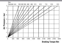
Maximum Pressure 7 bar Maximum Braking Force = 6.9kN @ 7 bar Weight of MR caliper and thruster - 7.82kg Weight of MR2 caliper and thruster - 8.32kg Weight of thruster only - 1.32kg Volume displacement of thruster at full stroke = 300
