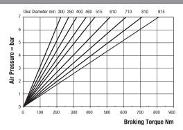
Maximum Pressure 7 bar Maximum Braking Force = 1.9kN @ 7 bar Weight of caliper and thruster - 7.3kg
