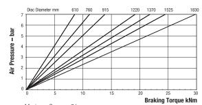
Maximum Pressure 7 bar Maximum Braking Force = 36kN @ 7 bar Weight of caliper and thruster - 40.8kg Weight of thruster only - 6.8kg Volume displacement of thruster at full stroke = 1.8 l
