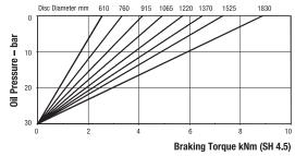
Maximum Braking Force SH 4.5: 10.5kN Minimum Pressure for full retraction: 38 bar Weight of caliper and thruster - 48.7kg Weight of thruster only - 14.7kg Volume displacement of thruster at full retraction = 56ml
