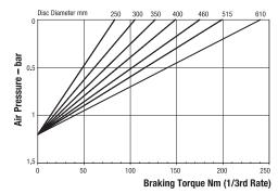
Maximum Braking Force 1/3rd rate: 0.87kN Minimum Pressure for full retraction: 1.7 bar Weight of caliper and thruster - 4.9kg Weight of thruster only - 3.4kg Volume displacement of thruster at full retraction = 950ml
