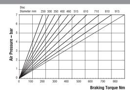
Maximum Pressure 7 bar Maximum Braking Force = 1.9kN @ 7 bar Weight of MR caliper and thruster - 6.8kg Weight of MR2 caliper and thruster - 7.3kg Weight of thruster only - 0.3kg Volume displacement of thruster at full stroke = 64ml
