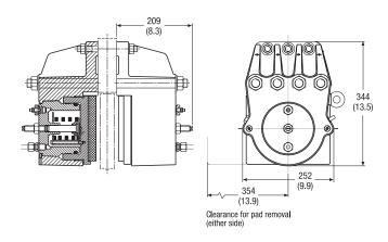
The Twiflex VKHD disc brake caliper is comprised of two halves, or hydraulic modules, and is suitable for use with a minimum disc thickness of 20mm. The modules are mounted each side of a central mounting plate 12mm thicker than the brake disc. Minimum disc diameter is 1000mm.
