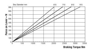
Weight of caliper and lever assembly - 10.62kg Weight of lever assembly only - 1.4kg Maximum Braking Force = 8.3kN @ 0.9kN force on lever
