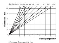
Maximum Prasking Force = 20kN @ 110 bar Weight of caliper - 5.82kg Volume displacement per 1mm stroke at each pad = 4.8ml
