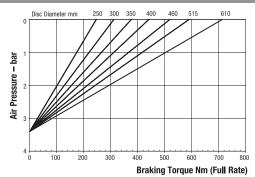
Maximum Braking Force full rate: 2.6kN Minimum Pressure for full retraction: 5 bar Weight of caliper and thruster - 4.9kg Weight of thruster only - 3.4kg Volume displacement of thruster at full retraction = 950ml
