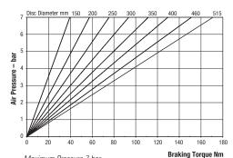
Maximum Pressure 7 bar Maximum Braking Force = 0.72kN@ 7 bar Weight of caliper and thruster - 0.8kg Weight of thruster only - 0.05kg
