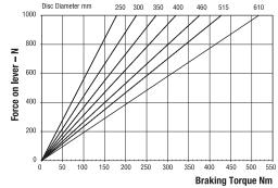
Maximum Braking Force = 1.88kN @ 0.8kN force on lever
