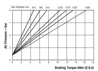
Maximum Braking Force S 8.4: 19.5kN Minimum Pressure for full retraction: 4.8 bar Weight of caliper and thruster - 46.2kg Weight of thruster only - 12.2kg Volume displacement of thruster at full retraction = 1.3 l
