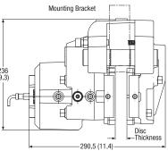
The Twiflex VCS-FL disc brake caliper comprises a single spring module forming the 'active' side of this floating unit and is available for use where space is limited or to accommodate axial disc float of ±6mm.
