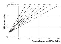
Maximum Braking Force 1/3rd rate: 0.87kN Minimum Pressure for full retraction: 17 bar Weight of caliper and thruster - 5.5kg Weight of thruster only - 4kg Volume displacement of thruster at 4mm retraction = 5ml
