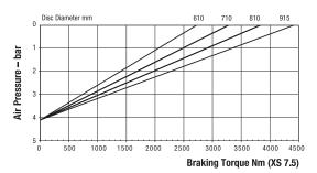
Maximum Braking Force XS 7.5: 11.2kN Minimum Pressure for full retraction: 5 bar Weight of caliper and thruster - 14.12kg Weight of thruster only - 4.9kg Volume displacement of thruster at full retraction = 1.19 l
