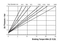
Maximum Braking Force S 12.9: 30kN Minimum Pressure for full retraction: 7 bar Weight of caliper and thruster - 48kg Weight of thruster only - 14kg Volume displacement of thruster at full retraction = 1.3 l
