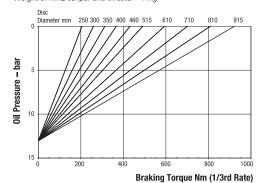
Minimum Pressure for full retraction: 17 bar Maximum Braking Force 1/3rd rate: 2.2kN Weight of MR caliper and thruster - 10.5kg Weight of MR2 caliper and thruster - 11kg
