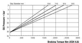
Maximum Braking Force XSH 4.6: 6.8kN Minimum Pressure for full retraction: 40 bar Weight of caliper and thruster - 13.22kg Weight of thruster only - 4kg Volume displacement of thruster at 6mm retraction = 9.1ml
