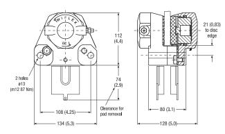
The standard Twiflex T20 disc brake caliper is split caliper design suitable for use with a minimum disc thickness of 12.7mm. Optionally, the caliper may be supplied in a modified form for use with a minimum disc thickness of 8mm. Normally the brake is side mounted, however, for use with a disc thickness greater than 20mm, the split design allows the modules to be mounted each side of a central mounting plate of the same thickness as the brake disc. Minimum disc diameter is 300mm.
