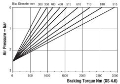
Minimum Pressure for full retraction: 3.1 bar Maximum Braking Force XS 4.6: 6.8kN Weight of caliper and thruster - 11.5kg Weight of thruster only - 4.5kg Volume displacement of thruster at full retraction = 1.19 l
