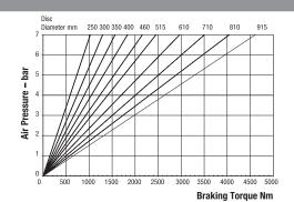
Maximum Pressure 7 bar Maximum Braking Force = 10.8kN @ 7 bar Weight of MR caliper and thruster - 8.56kg Weight of MR2 caliper and thruster - 9.06kg Weight of thruster only - 2.06kg Volume displacement of thruster at full stroke = 426ml
