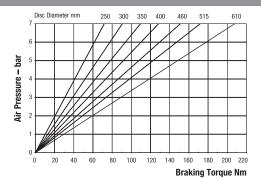
Maximum Pressure 7 bar Maximum Braking Force = 0.76kN @ 7 bar Weight of caliper and thruster - 1.89kg Weight of thruster only - 0.39kg Volume displacement of thruster at full stroke = 21ml
