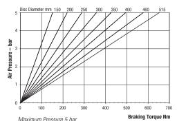
Maximum Braking Force = 2.75kN@ 5 bar Weight of caliper and thruster - 1.9kg
