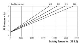
Maximum Braking Force XS 9.6: 14.3kN Minimum Pressure for full retraction: 6.5 bar Weight of caliper and thruster - 14.32kg Weight of thruster only - 5.1kg Volume displacement of thruster at full retraction = 1.19 l
