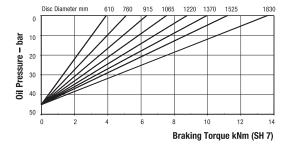
Maximum Braking Force SH 7: 16.5kN Minimum Pressure for full retraction: 59 bar Weight of caliper and thruster - 49.7kg Weight of thruster only - 15.7kg Volume displacement of thruster at full retraction = 56ml
