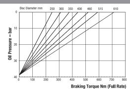
Maximum Braking Force full rate: 2.6kN Minimum Pressure for full retraction: 50 bar Weight of caliper and thruster - 5.5kg Weight of thruster only - 4kg Volume displacement of thruster at 4mm retraction = 5ml
