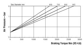
Maximum Braking Force XS 4.6: 6.8kN Minimum Pressure for full retraction: 3 bar Weight of caliper and thruster - 13.72kg Weight of thruster only - 4.5kg Volume displacement of thruster at full retraction = 1.19 l
