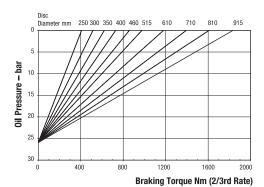
Minimum Pressure for full retraction 33 bar Maximum Braking Force 2/3rd rate: 4.3kN Weight of MR caliper and thruster - 10.5kg Weight of MR2 caliper and thruster - 11kg
