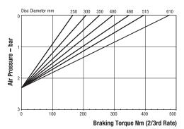
Maximum Braking Force 2/3rd rate: 1.74kN Minimum Pressure for full retraction: 3.3 bar Weight of caliper and thruster - 4.9kg Weight of thruster only - 3.4kg Volume displacement of thruster at full retraction = 950ml
