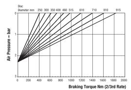
Minimum Pressure for full retraction: 3.3 bar Maximum Braking Force 2/3rd rate: 4.3kN Weight of MR caliper and thruster - 10.0kg Weight of MR2 caliper and thruster - 10.5kg
