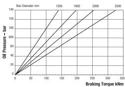
Maximum Pressure 140 bar Maximum Braking Force = 285kN @ 140 bar Weight of caliper - 287kg Volume displacement per 1mm stroke at both pads = 51.7ml
