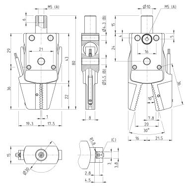
A = port connection B = mounting hole C = sensor groove
