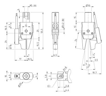
A = connection port B = mounting hole C = sensor groove
