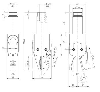
A = connection port B = fixing thread C = sensor fixing hole
