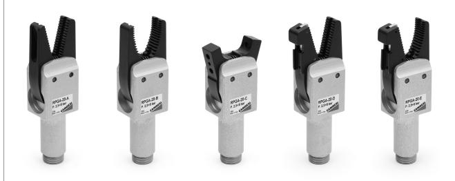
Thanks to a piston with a size of 20mm and to the direct transfer of the force from the piston to the fingers, Series RPGA guarantees a strong and a safe grip. Their technical features ensure a high gripping force and make these grippers particularly suitable in the removal of injection molded items.
