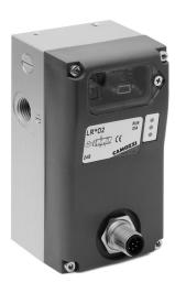
Series LR digital proportional servo valves are direct driven 3/3-way valves with a patented rotating spool system with closed loop control circuit. The electronic board is integrated into the valve's body ready to connect.
